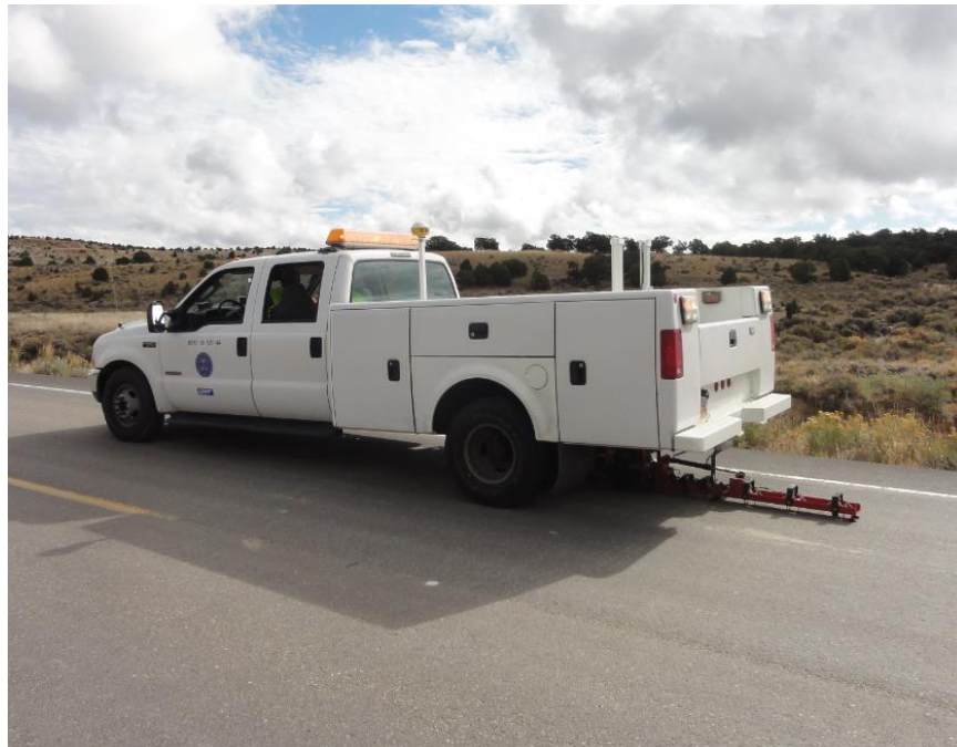
Figure 3-2: FWD testing of pavement structure.
